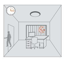
If there is no more movement, the light turns off automatically after hold-time preset.
